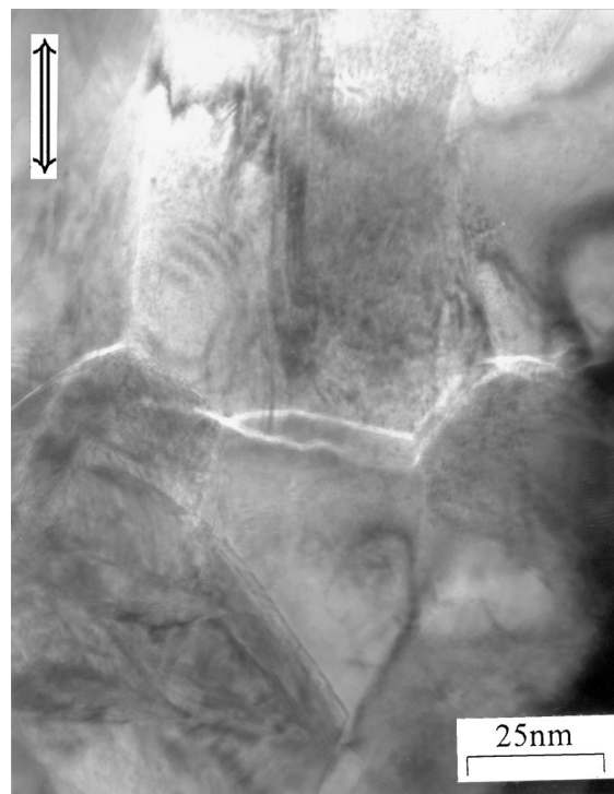
Figure 3 TEM micrograph of a specimen tested at 1823 K, 2 \times 10^{-2} \text{ s}^{-1} , showing intergranular cracks seen as white features at mid-section of the photograph; arrows indicate tensile direction.
